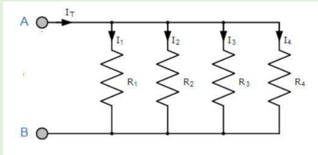
R1 can be replaced with 4 resistors in parallel of 10k each.
