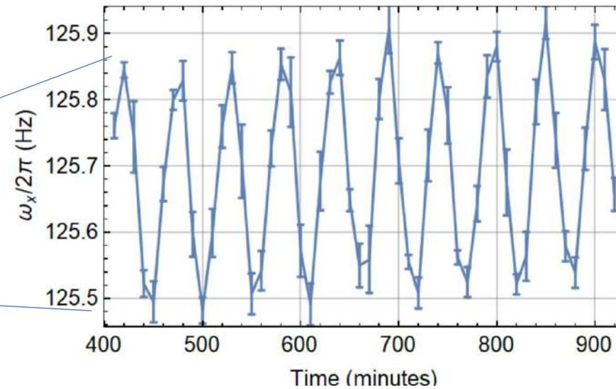
Frequency stability limited by 3 degree C room temperature fluctuation
