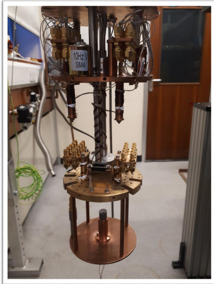
300 mK plate construction of the He-3 insert of the cryostat at Southampton. Visible are SQUID detector above a lead trap at the bottom plate of the 300 mK assembly, as well as a geophone sensor for reference measurements of vibrational noise at the 1 K plate. Also visible are wire connectors all the way down to the 300 mK plate for the optional assembly of a Paul ion trap at the cryostat. Credits: UoS
