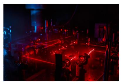
Photo of a 650nm laser beam path used to laser-cool barium ions. Photo by Lars Kruse, AU
