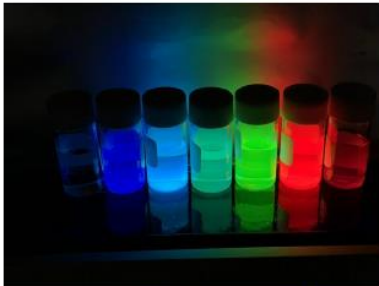
Some cesium lead halide ( \text{CsPbX}_3 ) nanocrystal dispersions made during my internship at IIT Genova, where the halide goes from chloride (left) to bromide (middle) to iodide (right) and mixtures thereof. Credits: J. Mulder.
